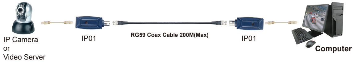
Passive IP Extender over Coax Cabling
