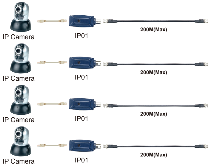
4 IP Cameras over Coax Cabling Solution
